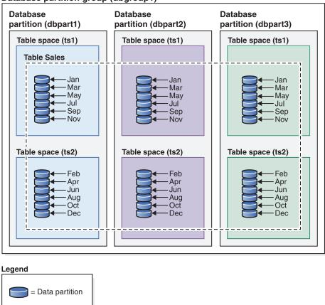
Figure 4. Demonstrating the complementary organization schemes of database partitioning and table partitioning. A table representing monthly sales data is partitioned into multiple data partitions, spanning two table spaces (ts1 and ts2) that are distributed across multiple database partitions (dbpart1, dbpart2, dbpart3) of a database partition group (dbgroup1).
