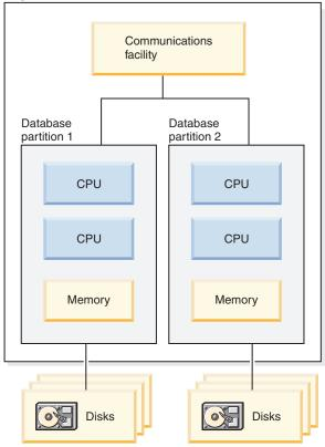
Figure 35. Partitioned database with symmetric multiprocessor environment
