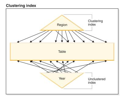
Figure 8. A regular table with a clustering index
