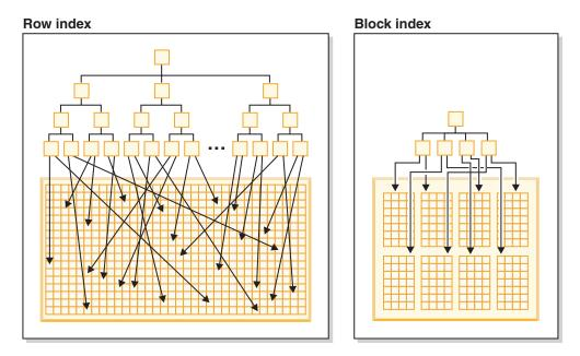
Figure 13. How row indexes differ from block indexes
