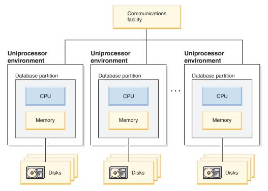
Figure 33. Massively parallel processing (MPP) environment
