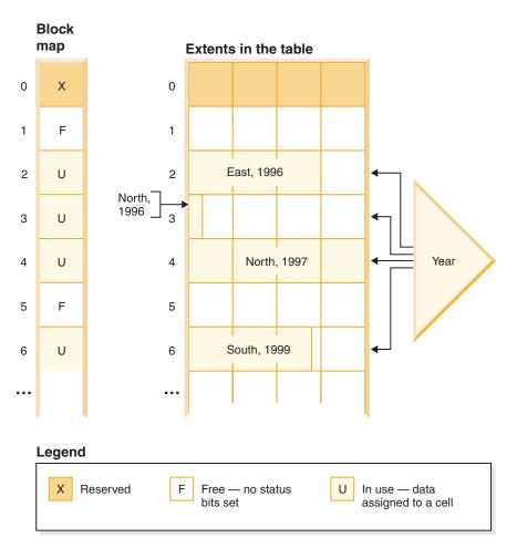
Figure 25. How a block map works
