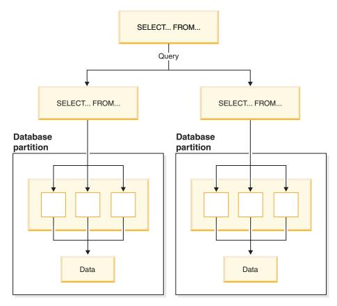
Figure 30. Simultaneous interpartition and intrapartition parallelism
