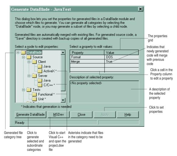
Figure 4-2. Generate DataBlade Dialog Box
