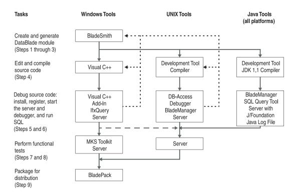
Figure 1-1. DataBlade Module Development Cycle
