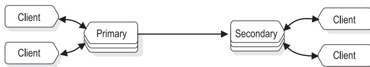
Figure 20-2. A primary and secondary database server in a data replication configuration
