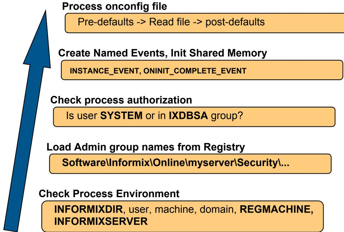
Figure 13 Oninit process initialization sequence
