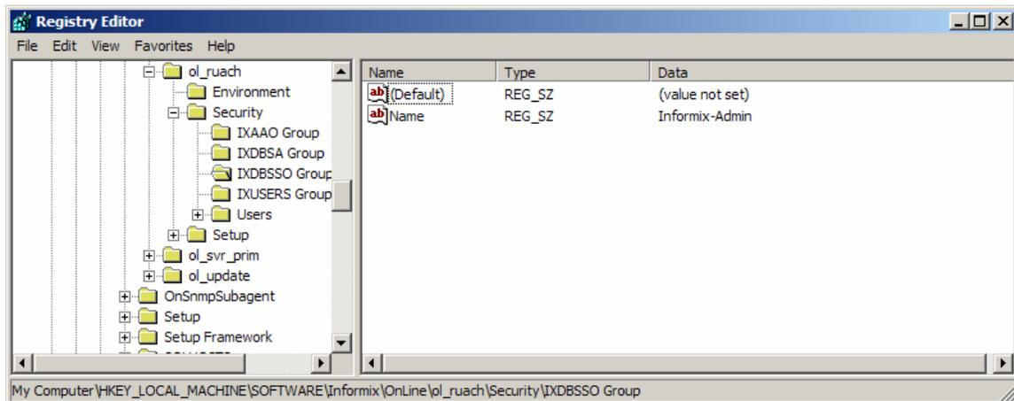
Figure 5 An IDS instance registry sub-key showing the security settings
