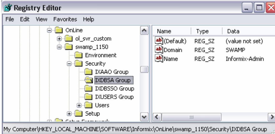
**Figure 3** An IDS instance registry sub-key showing the IXDBSA Group
