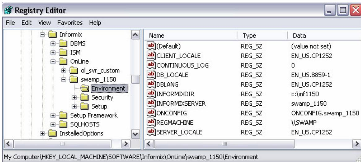
Figure 4 An IDS instance registry sub-key showing the environment settings
