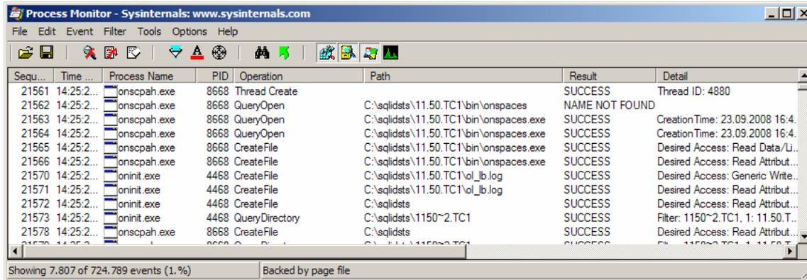
Figure 24 Part of Process Monitor output for IDS startup
