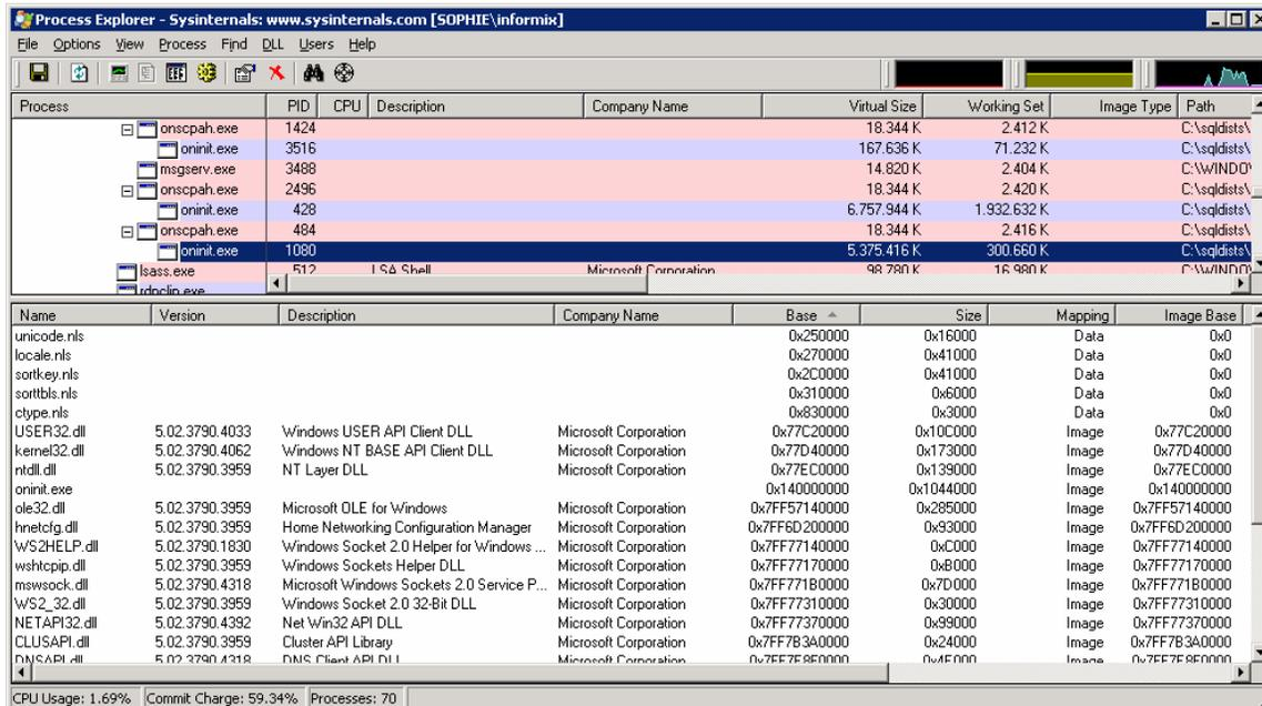
Figure 9 Process Explorer displaying 64-bit DLL load addresses for oninit.exe
