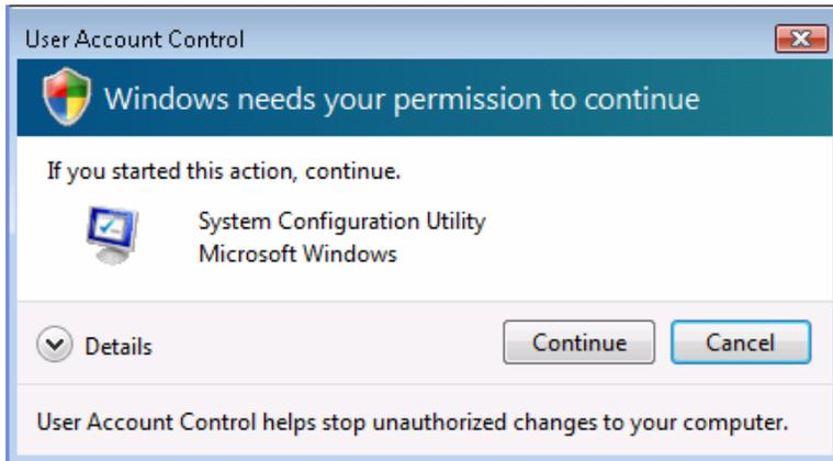
**Figure 20 Windows prompts for a trusted program asking to run with elevated privileges**
