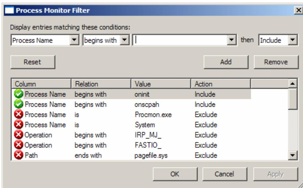
Figure 23 Setting up a Process Monitor filter for IDS
