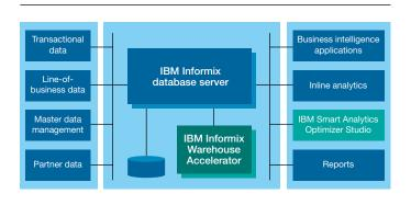
Figure 1: Informix Warehouse Accelerator architecture
