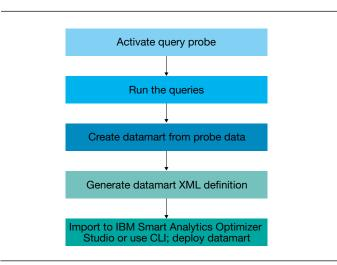
*Figure 5*: Informix contains a built-in tool to help you create a datamart in five steps.
