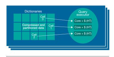
Figure 11: Efficient parallel scanning for query processing
