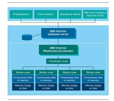
Figure 2: Sample architecture with one coordinator node and four worker nodes
