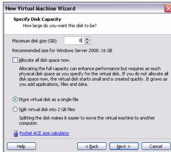
Figure 12-24 Specify Disk Capacity window
