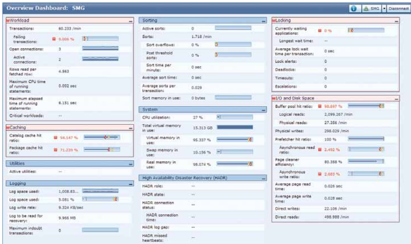
Figure 1: The InfoSphere Optim Performance Manager dashboard has a color-coded, web-based interface designed to quickly alert users to problematic areas. Once a problem has been identified, specific diagnostics and details are provided to focus on that area. Integration with InfoSphere Optim products provides the resolution needed to correct the problem.
