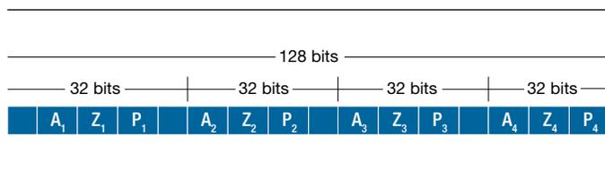
Figure 9: Loading column values into processor registers
