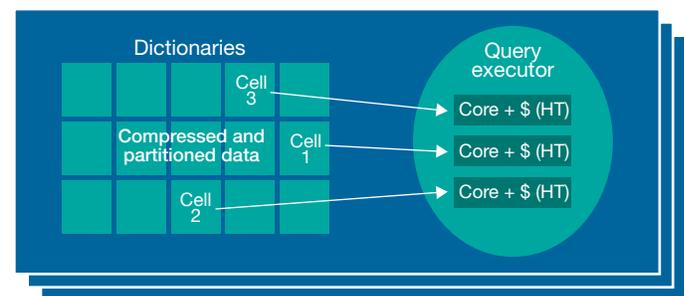
Figure 11: Efficient parallel scanning for query processing
